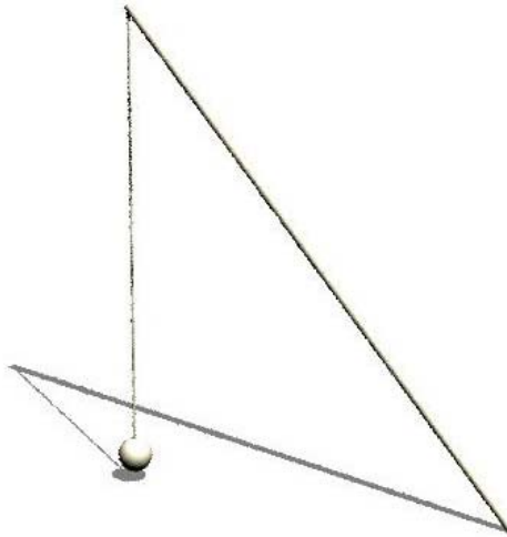
Setting out to north using a pole and plumb-bob
