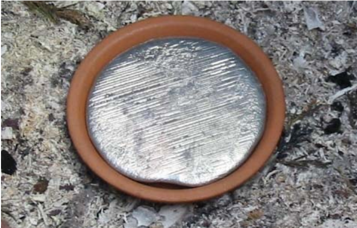
Cast tin after cooling
