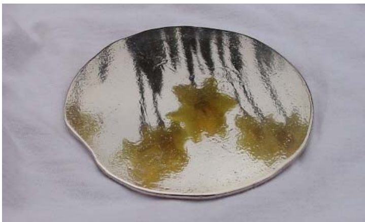
Cast tin after hand polishing using chalk paste
